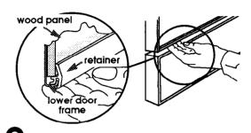
9. Important: Run fingers along bottom of retainer to check that retainer is lower that the lower door frame.
